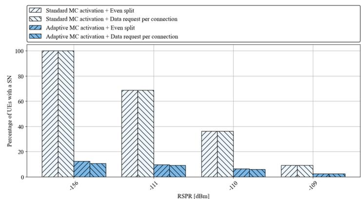
Fig. 1. Percentage of UEs with a SN for different SN addition thresholds.
