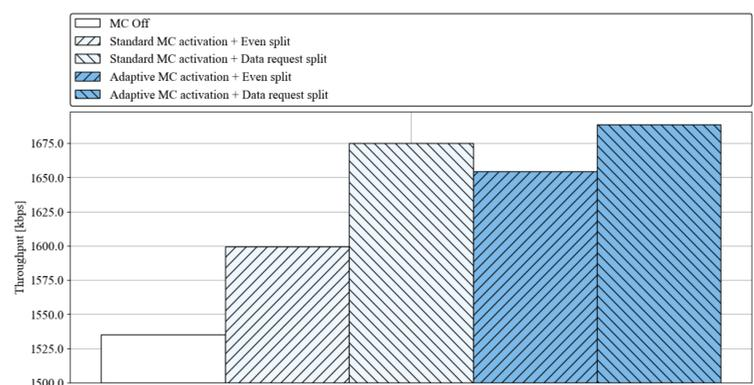
Fig. 2. Average per user throughputs with -111 dBm SN addition threshold.
