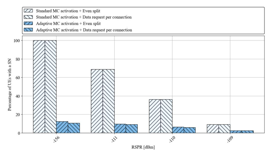
Fig. 1. Percentage of UEs with a SN for different SN addition thresholds.
