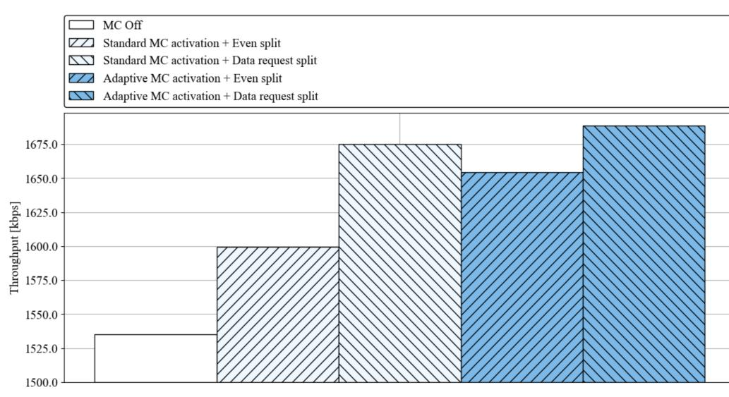
Fig. 2. Average per user throughputs with -111 dBm SN addition threshold.
